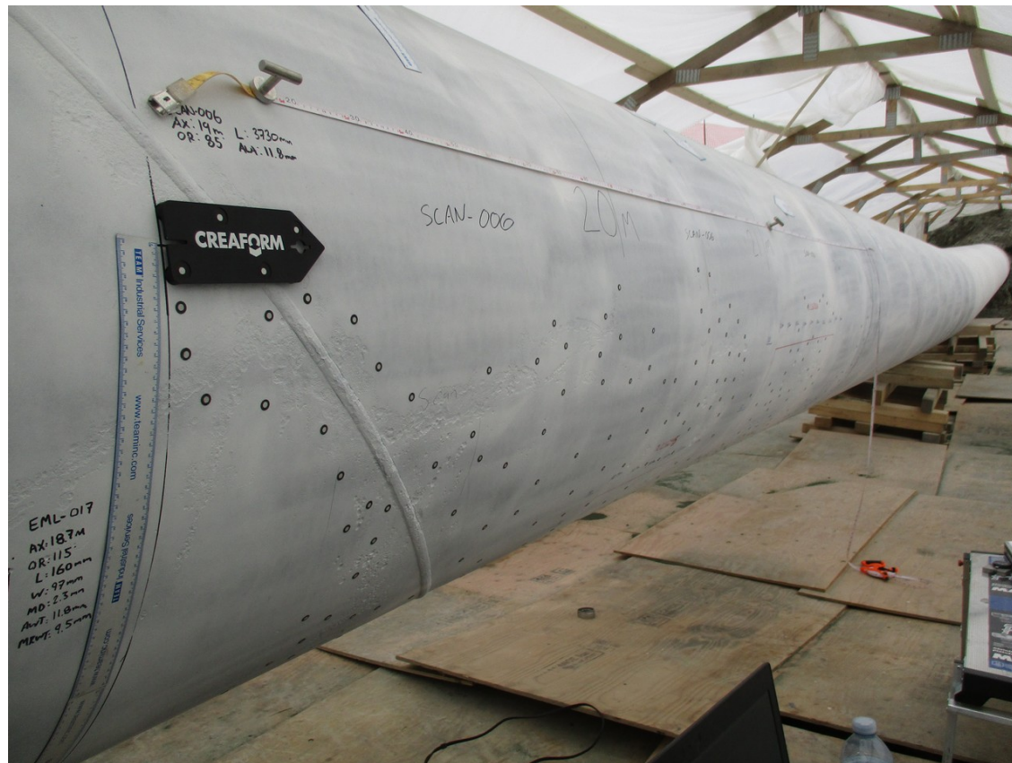
Figure 10: Field laser Scanning Corrosion feature
