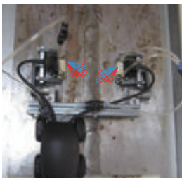
Dual-side Butt Weld Inspection
