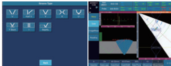
Flat weld solution including various weld types, raytracing capability and overlay help to locate the flaw position visually.
