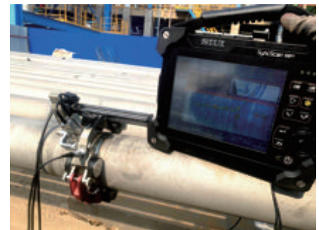
Austenitic weld inspection
