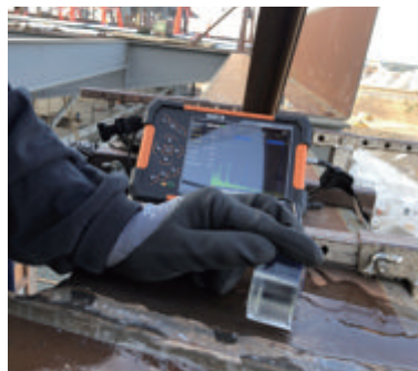
Ultrasonic weld inspection
