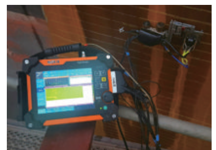
PA corrosion solution
