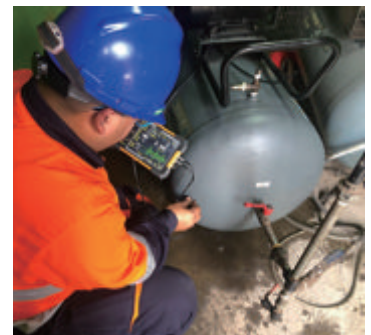
Ultrasonic thickness measurement
