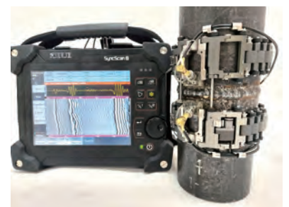
LPS-02/08 are compatible with TOFD probes.
