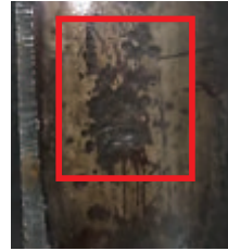
C-scan for pipe scattered spot corrosion
