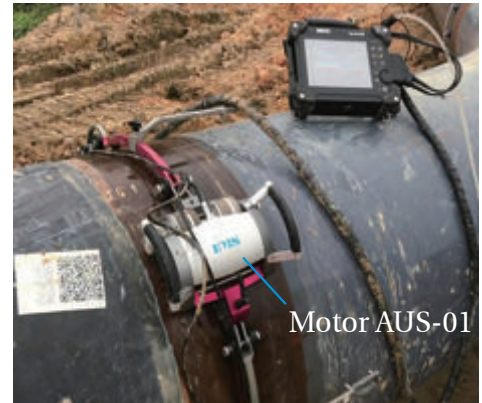
With motor AUS-01 for automatic scanning
